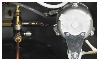
Integrated fluid pump: For charging high-volume A/C systems
